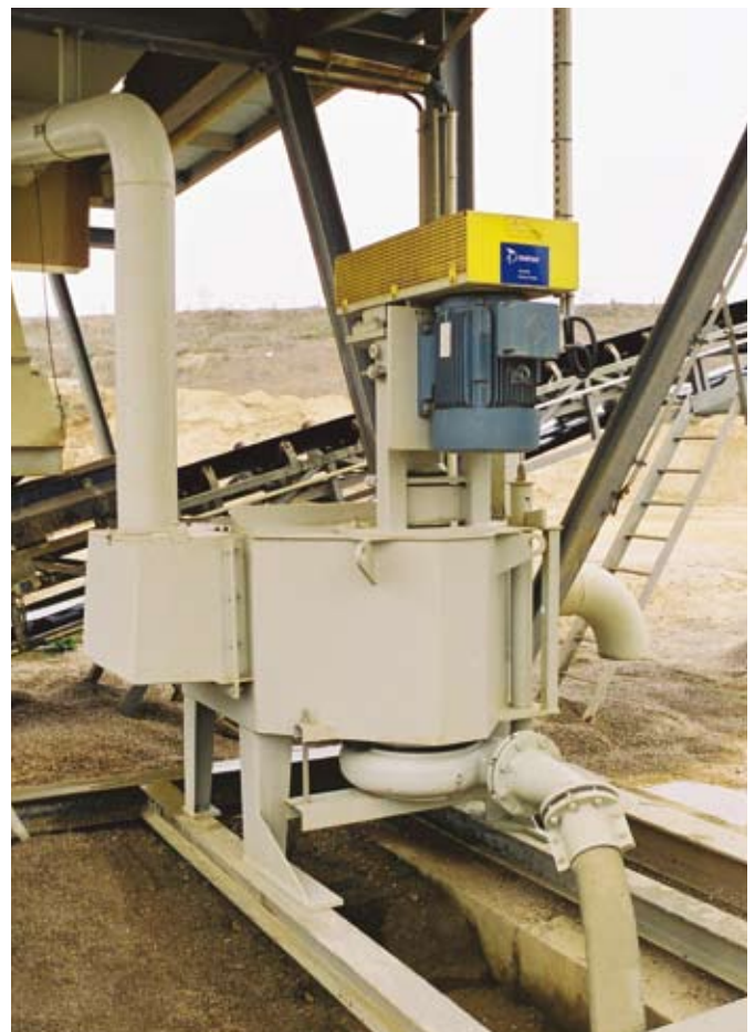
VT 150 customer adjusted for cyclone feed application in a sand plant.
