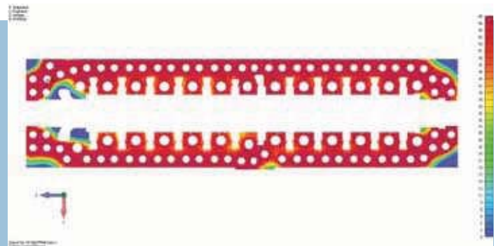
Fig 1. Result of FEA of packing under a test pressure of 276 bar. No leaking was found.
