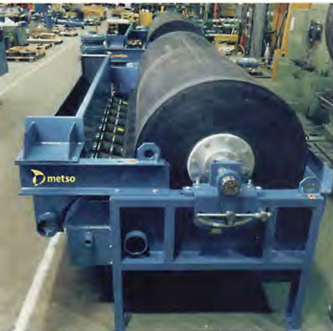
Wet magnetic separator before shipment to an North American iron ore operation.
