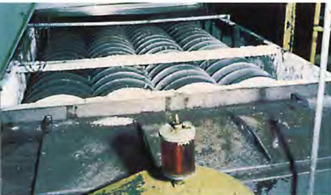
Holo-Flite® processor is used to cool sodium tripolyphosphate in a chemical plant.
