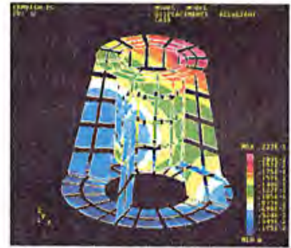
The finite element method has been used to check that the adequate rigidity has been achieved in the design.
