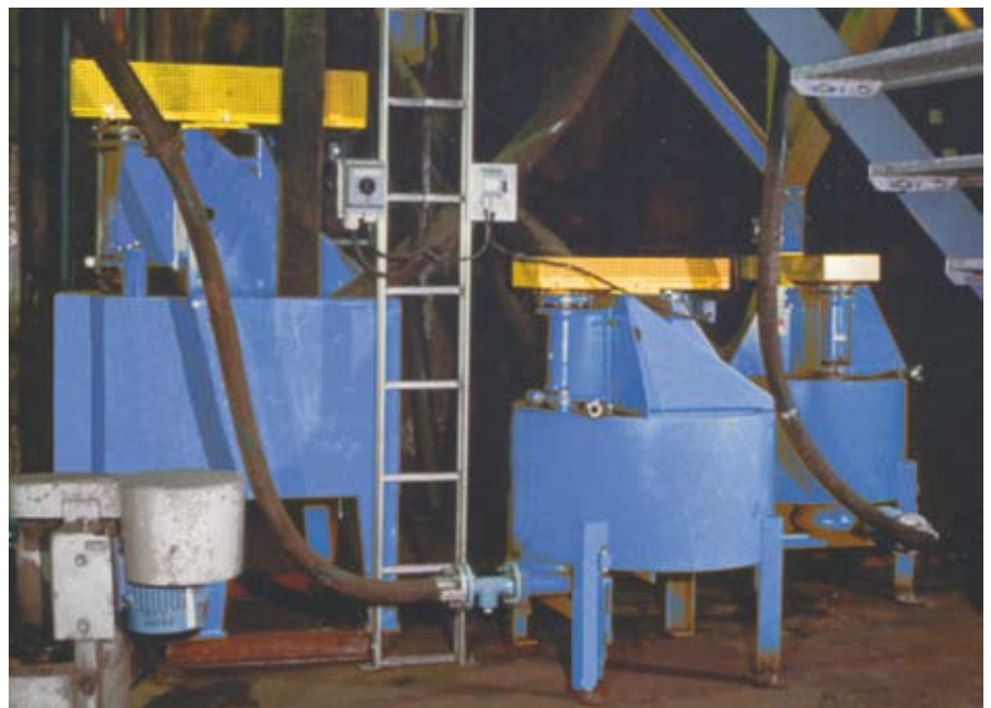
Metso VT pumps for pumping of concentrate, middlings and tailings from spirals for treatment of slag <2 mm.
