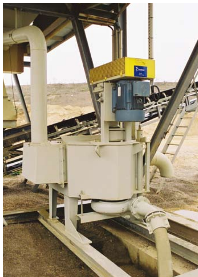
VT 150 customer adjusted for cyclone feed application in a sand plant.
